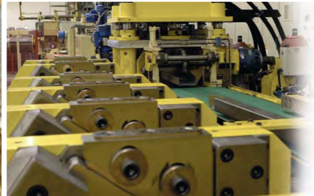
High-speed roll-forming technology is used in the production of Link 51's XL pallet racking beams.
